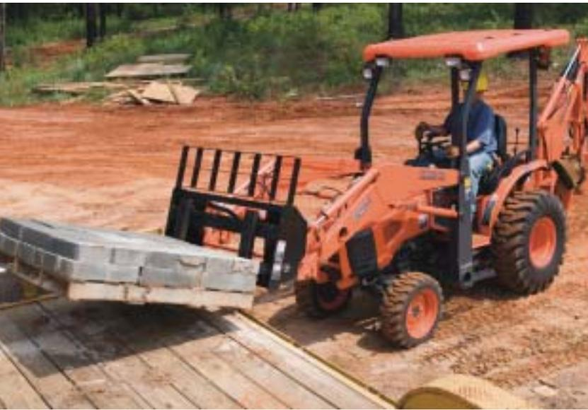
Implements are the key to getting the most out of your B26 tractor/loader/backhoe. Remove the backhoe and attach our 3-point hitch to use a slasher, rotary hoe, rotary cutter, power rake and other PTO-driven implements. Or use our Skid Steer-type quick coupler to attach implements like a pallet fork or bale spear to the front.
