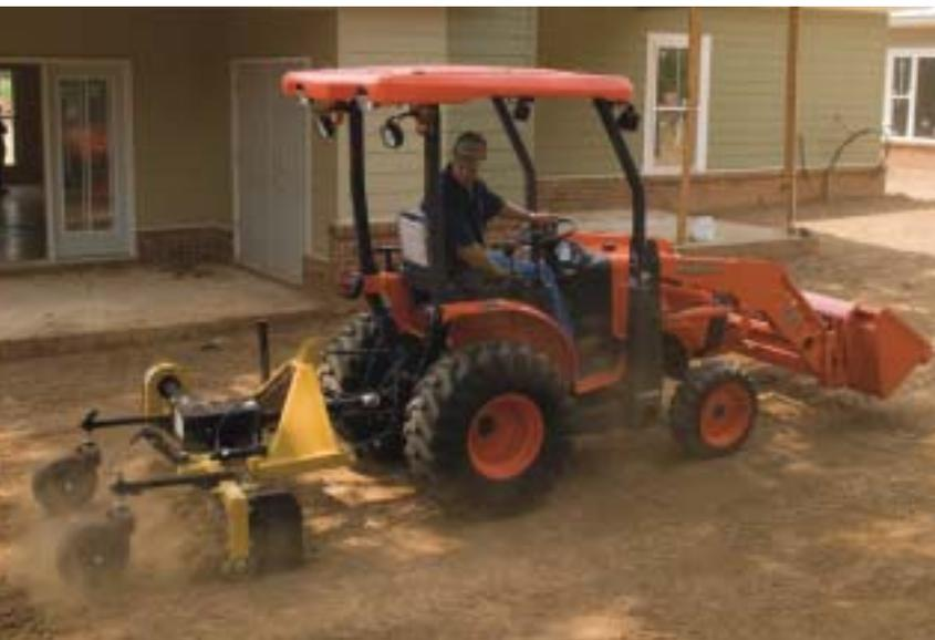
Built specifically for loader and backhoe applications, the B26 features an integrated main frame to ensure durability. Its 26HP engine provides high power and torque rise as well as low noise. And, a 3-point hitch greatly improves the B26's versatility.
